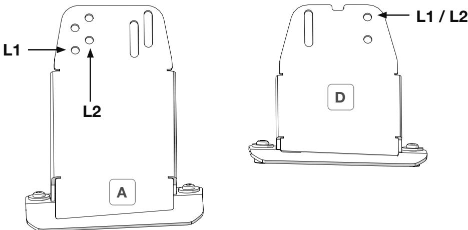
**EN** Position the bracket and awning so that they do not interfere with the side door.
